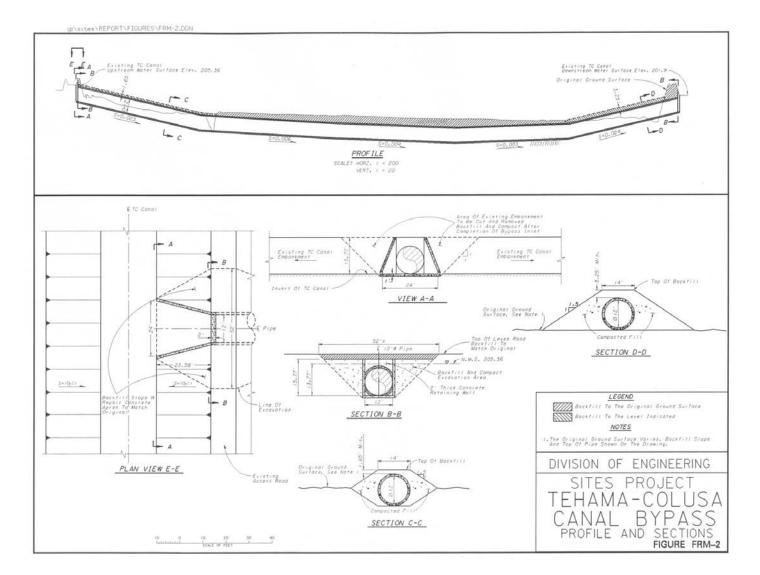
Figure B.3-36. Tehama-Colusa Canal Bypass – Profile and Sections
