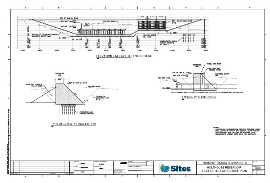
Figure B.3-34. Holthouse Reservoir Concrete Dam
