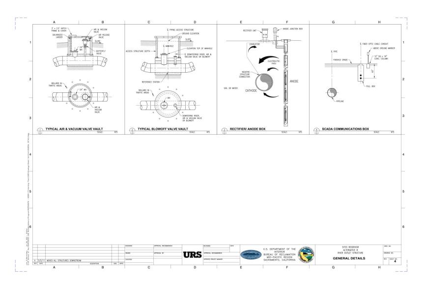
Figure B.3-40. Typical Pipeline Air Valve and Blow-off Details
