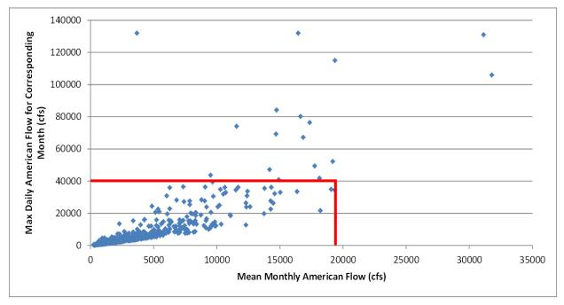
Figure 11N-2. Relationship between Mean Monthly Flows and Maximum Daily Flows during December through April, American River Downstream of Hazel Avenue, 1950–2015. Minimum monthly flow is identified in red.
