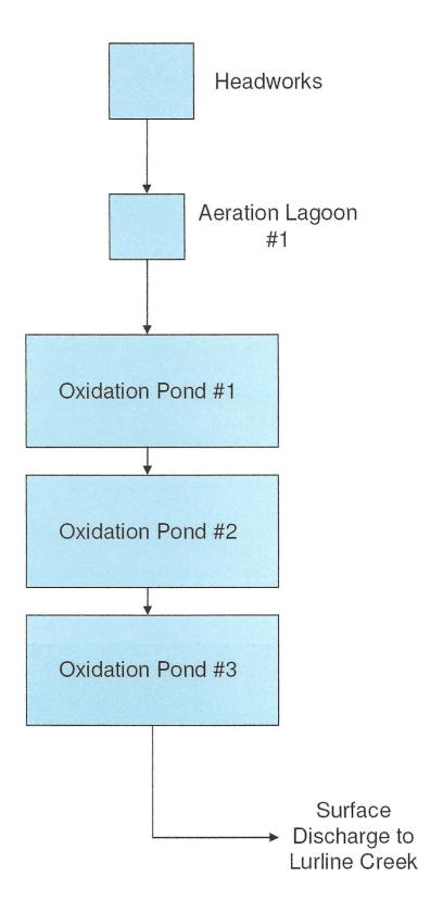
Figure 1a: Process Flow Diagram of Existing WWTF
