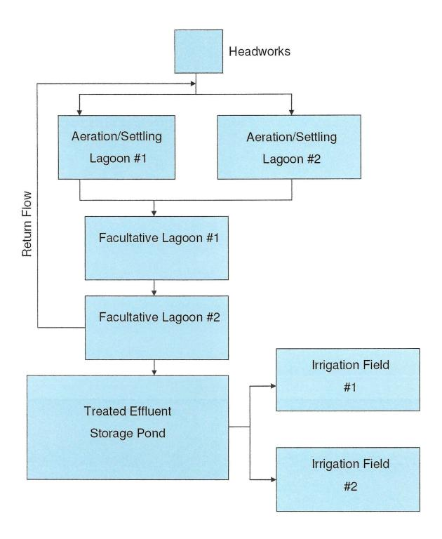
Figure 1b: Process Flow Diagram of Proposed WWTF
