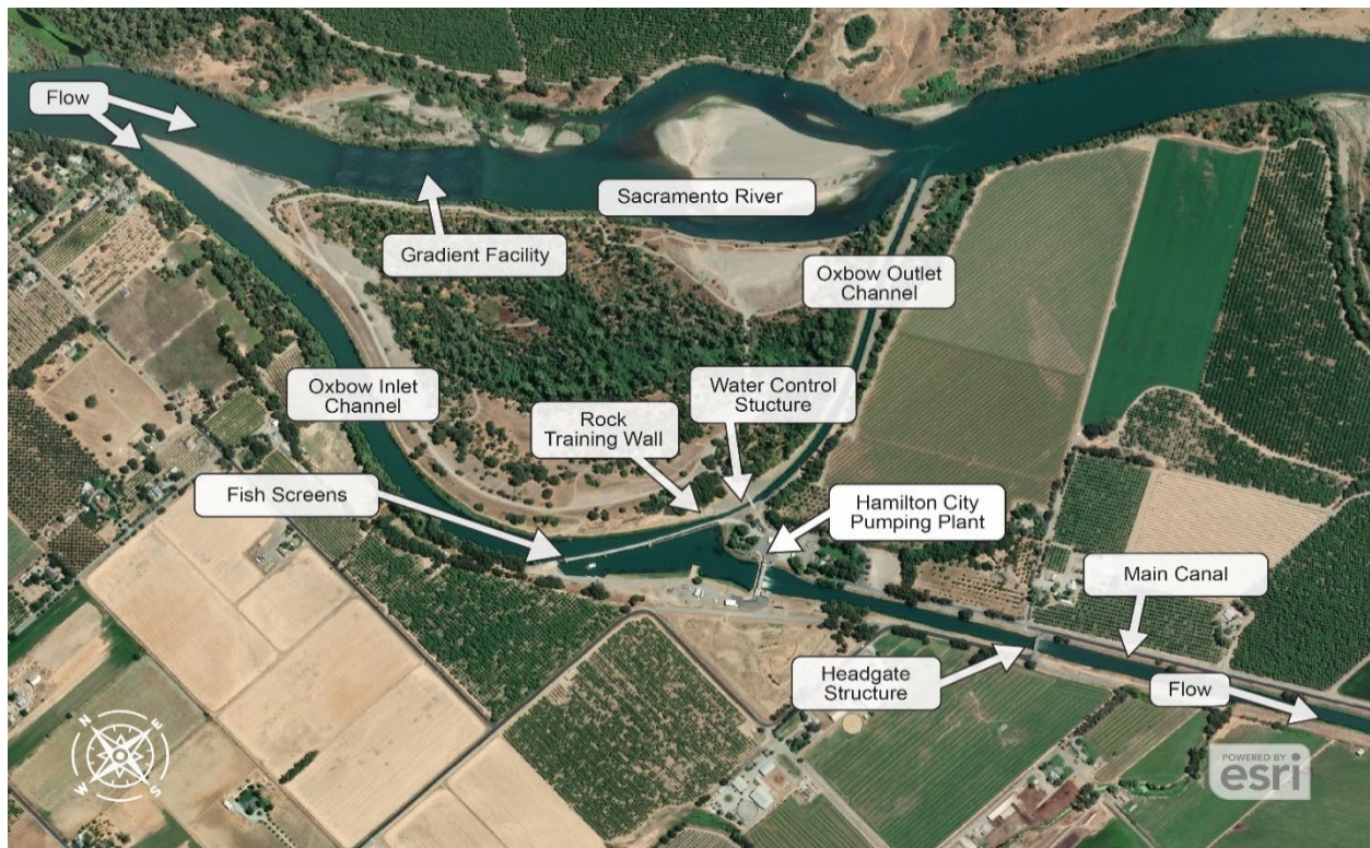
Figure 2. GCID HCPP Diversion Facility
