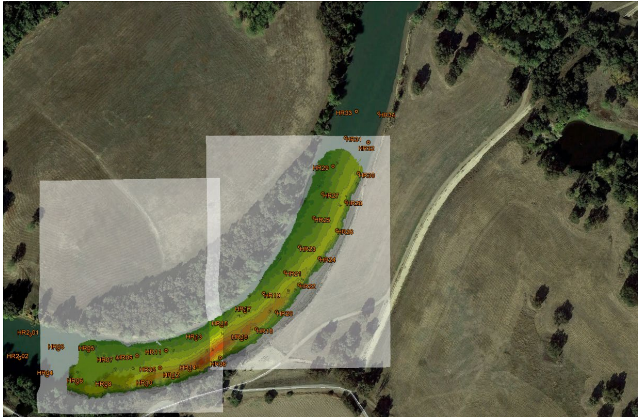
Figure 2 - Aerial photograph showing the bathymetry and hydrophone locations in study area
